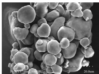
图6 番茄红素微胶囊扫描电镜图(× 600) Fig.6 Scanning electron microscope micrograph of lycopene microcapsule (× 600)
